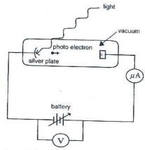
Using this apparatus it is found that light of wavelength 254 nm ejects photoelectrons from a silver plate. The work function of the silver surface is 4.7 eV.
