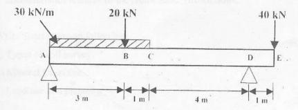
In the diagram shown above, the beam ABCDE is simply supported at points A and D. The beam carries a uniformly distributed load of 30 kN/m between the points A and C and concentrated loads of 20 kN and 40 kN at the points B and E, respectively.
