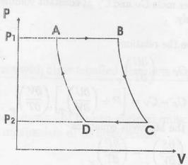
The Joule cycle shown above consists of two constant-pressure step connected by two adiabatics. Show that the Thermal efficiency of a reversible engine operating in this cycle, with an ideal gas of constant heat capacities as the working medium is
