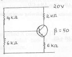
For the above npn transistor circuit find
